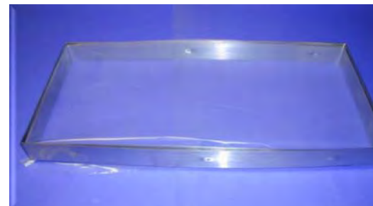
Partially assembled with sheet ready to be captured between 'bands'
