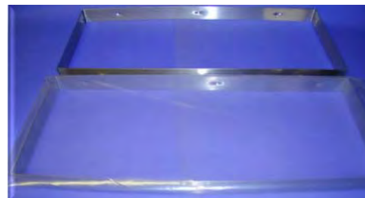
Partially assembled with sheet ready to be captured between 'bands'
